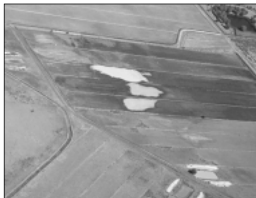
Improving water use efficiency can result from better managing factors such as water application and prevent symptoms of poor irrigation as shown here.
