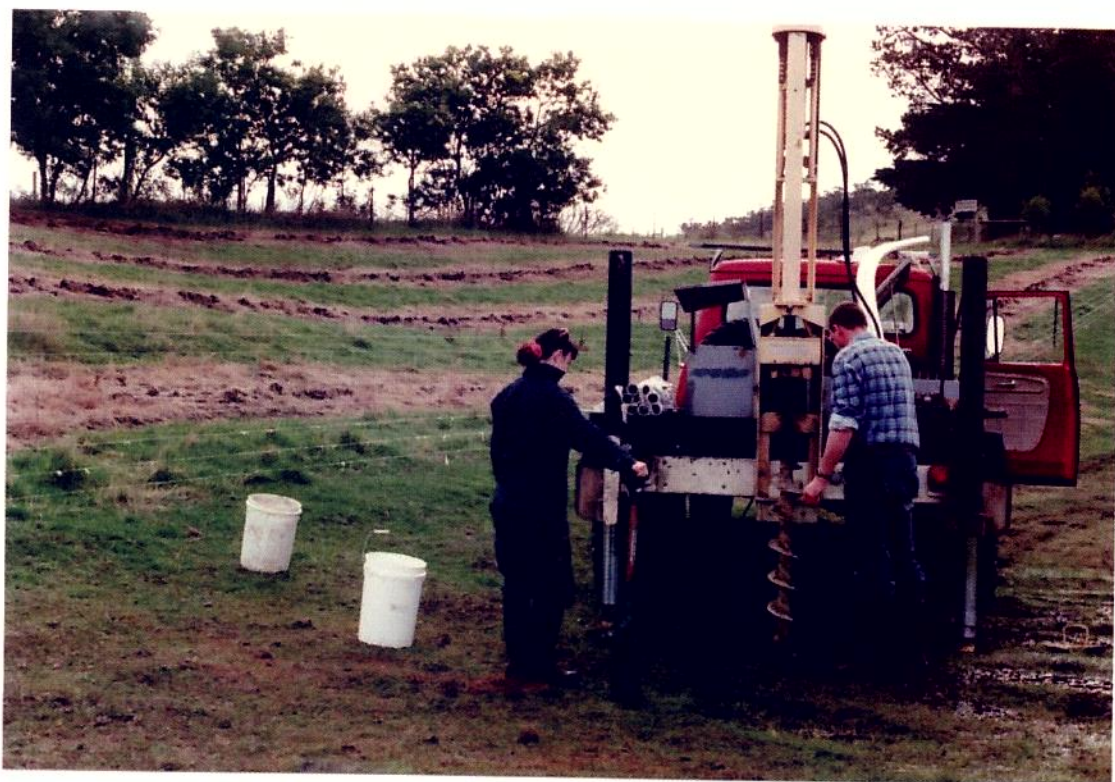
Plate 11. (extra to sub project 8) DPIF staff drilling for shallow bore installation to measure water table level and salinity next to tree planting.
