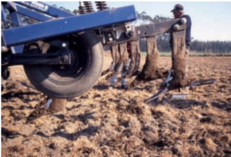
Figure 15. Winged rippers achieve the optimum soil shatter.
