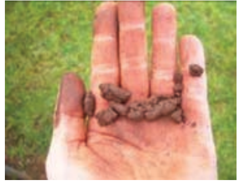
Figure 11b. At the optimum moisture content the soil sample will crack and break into short lengths.
