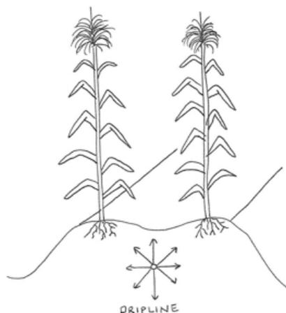
**Figure 2:** SDI location in centre of raised beds and direction of water movement
